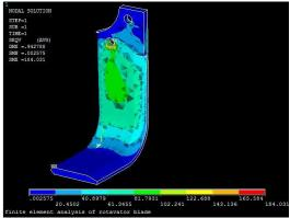
Fig. 3.3 Von mises stress for High carbon steel (9 mm thickness)
