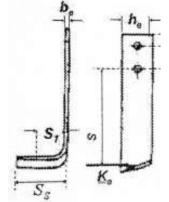
Fig. 2.2 Dimensions of the blade [11]
