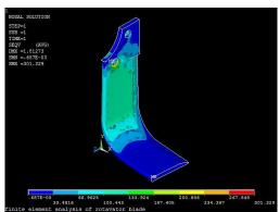
Fig. 3.2 Von mises stress for High carbon steel (8 mm thickness)
